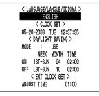
3 Press the [♥] or [▲] button to select "MODE" under <DAYLIGHT SAVING>.
